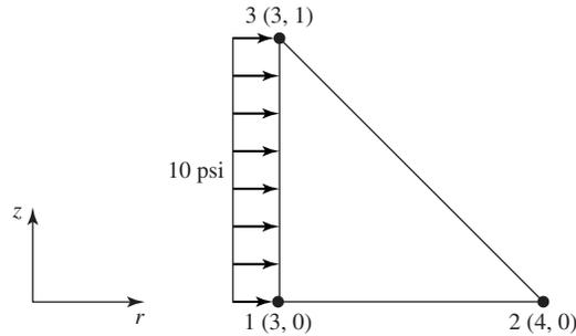
**Figure 9.11** Uniform radial pressure.
