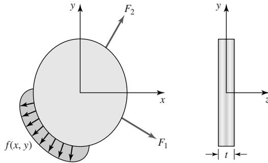
**Figure 9.1** An illustration of plane stress conditions.
