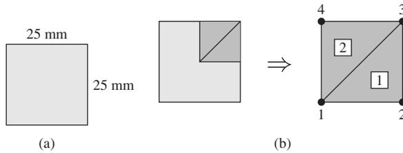
Figure 9.14 Finite element model of Example 9.7.
