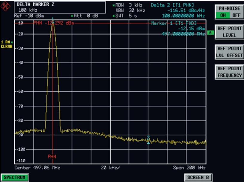
Fig. 6-2 Marker function for easy phase noise measurement
