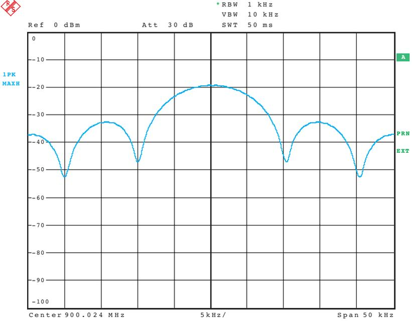
**Fig. 6-10** Real representation of envelope spectrum with a spectrum analyzer
