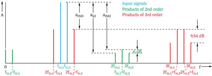
Fig. 5-7 Output spectrum of nonlinear network with two-tone input (magnitude spectrum)
