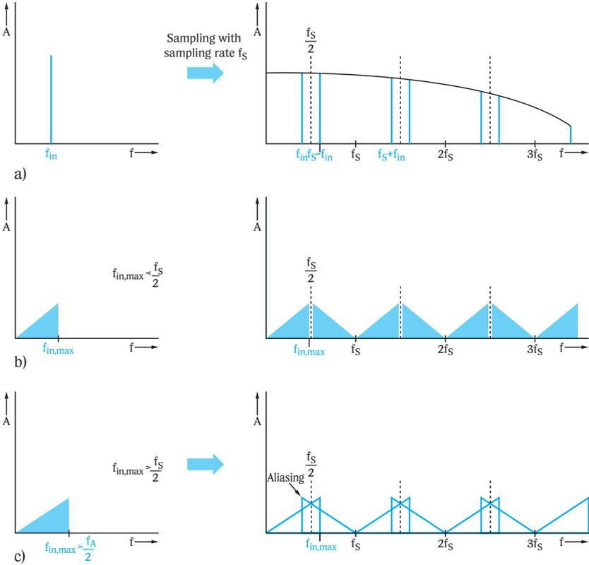
**Fig. 3-1** Sampling a lowpass filter with sampling rate  $f_s$
