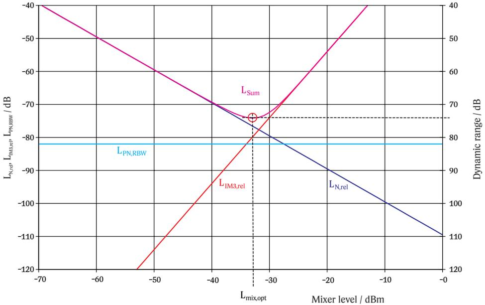
**Fig. 5-20** Dynamic range taking into account thermal noise, phase noise and 3rd order intermodulation products ( $NF = 24.5$  dB,  $IP3_{in} = 7$  dBm,  $L(f_{off}) = -122$  dBc (1Hz),  $B_{N,IF} = 10$  kHz)
