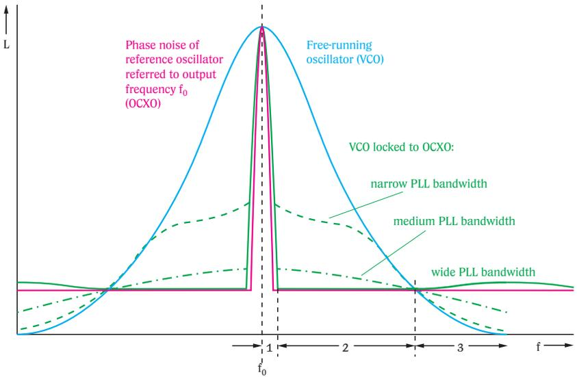
Fig. 5-11 Phase noise of OCXO, VCO and of VCO locked to OCXO at different PLL bandwidths
