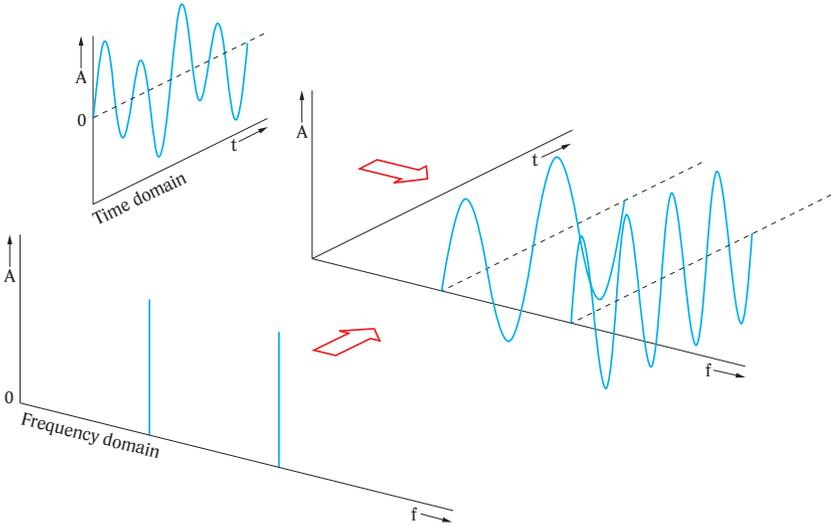
Fig. 2-2 Signals examined in time and frequency domain
