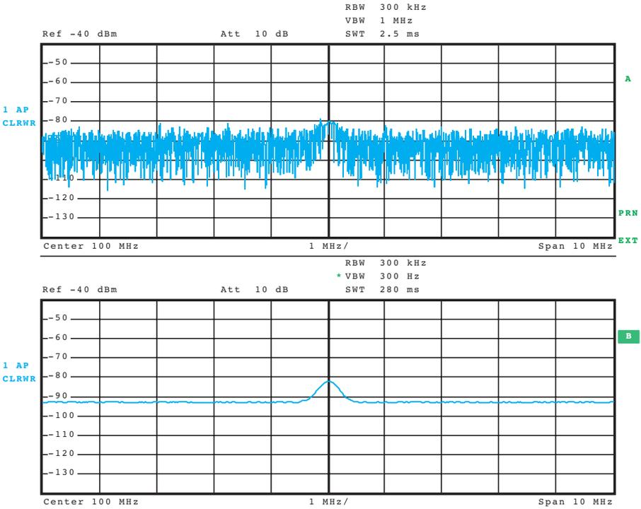
**Fig. 4-19** Sinusoidal signal with low S/N ratio shown for large (top) and small (bottom half of screen) video bandwidth
