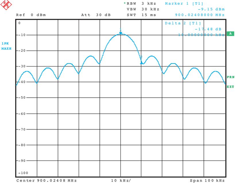
**Fig. 6-14** Envelope spectrum of pulsed signals
