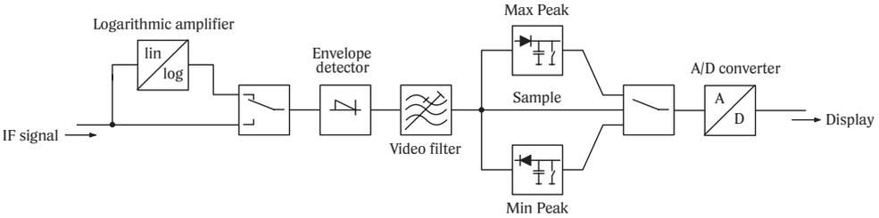
Fig 4-22 Analog realization of detectors
