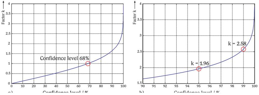
**Fig. 5-27** Coverage factor  $k$  as a function of confidence level
