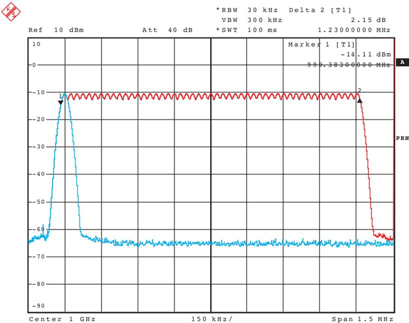
Fig. 6-23 Channel power measurement using integrated bandwidth method
