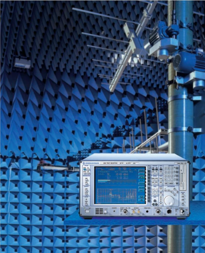
The designation as a "test receiver" is somewhat deceptive, since the ESI actually is a full-featured and high-grade spectrum analyzer. As a one-box solution for EMI compliance measurements, it provides all the functions required for EMI measurements conforming to standards. The ESI performs measurements to all relevant commercial and military standards, and its upper frequency limit of 40 GHz covers all frequency ranges that are significant for EMC measurements.
