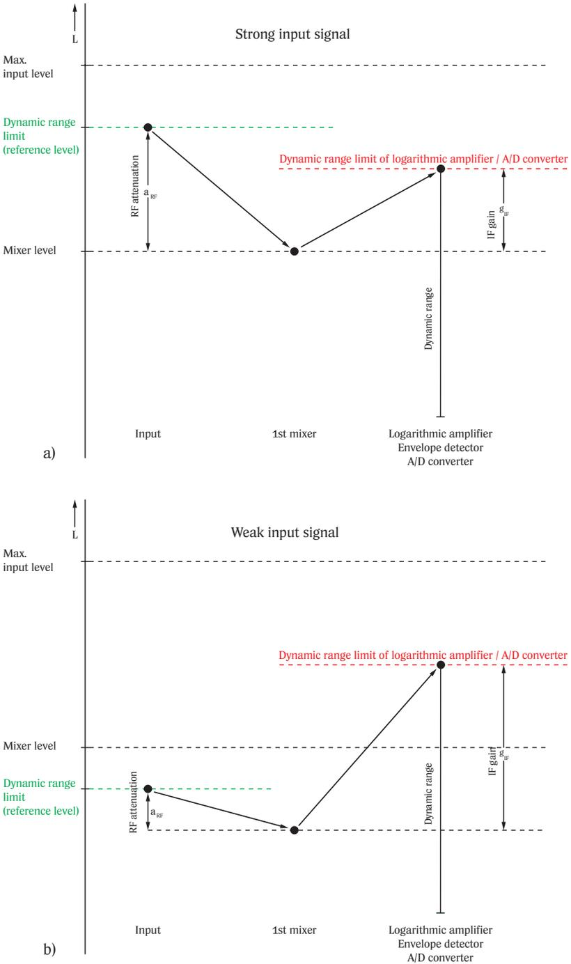
Fig. 4-30 Adaptation of RF attenuation and IF gain to maximum signal level to be displayed (max. signal level = reference level)
