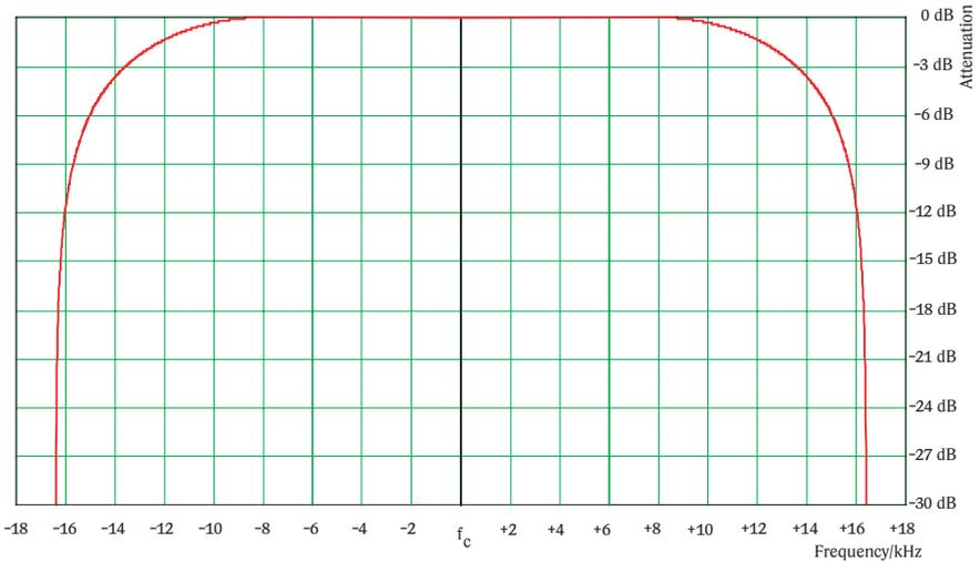
Fig. 6-24 Channel filter for IS-136 (NADC) systems
