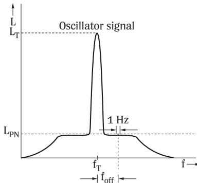
Fig. 6-1 Definition of SSB phase noise
