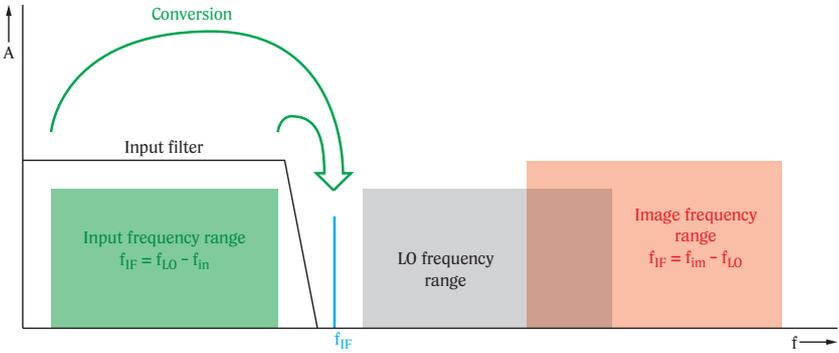
Fig. 4-4 Principle of high intermediate frequency
