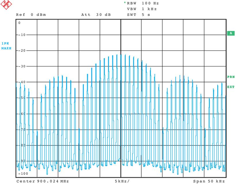
**Fig. 6-11** Real representation of line spectrum with a spectrum analyzer,
