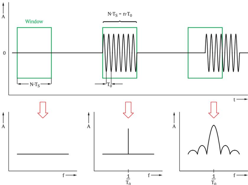
**Fig. 3-7** FFT of pulsed signals.
