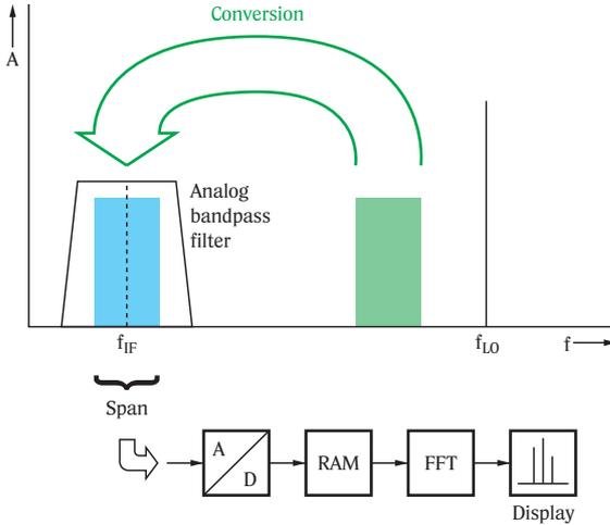
Fig. 4-14 Spectrum analysis using FFT
