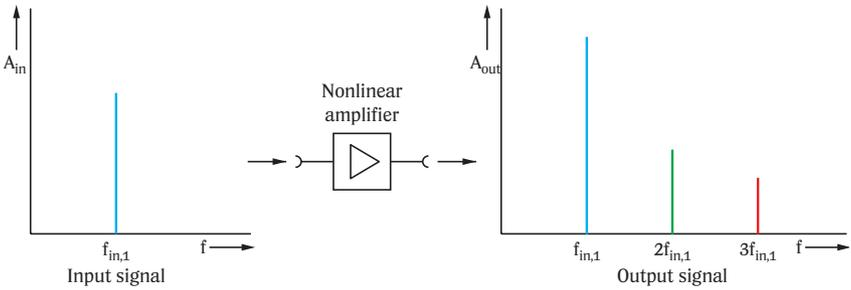
Fig. 5-5 Spectrum before and after nonlinear network
