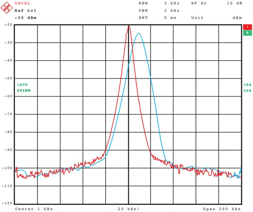
Fig. 4-29 Amplitude loss if minimum sweep time required is not attained (blue trace)
