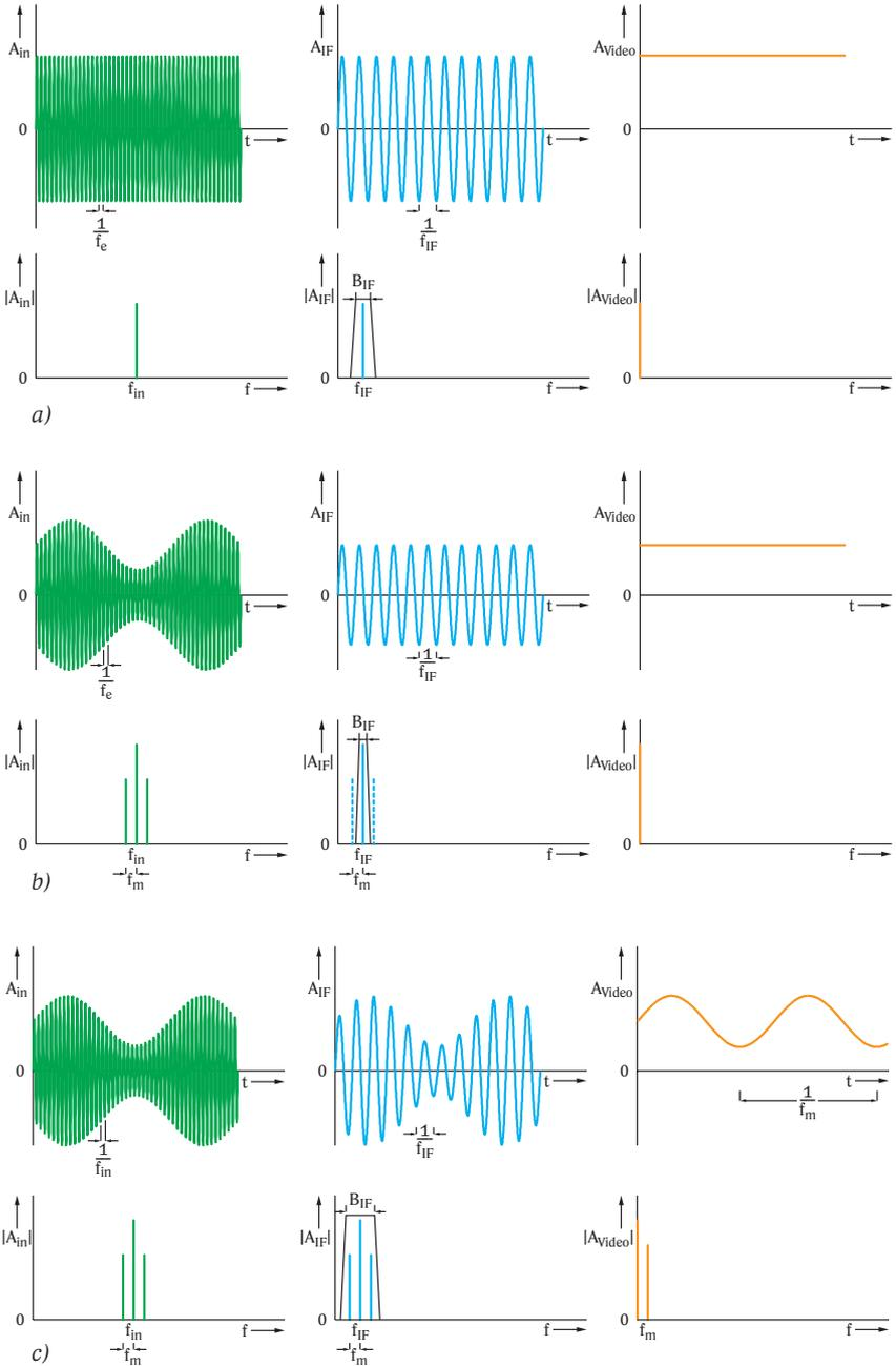
**Fig. 4-18** Video signal (yellow trances) and IF signal after IF filter (blue traces) for various input signals (green traces) and resolution bandwidths
