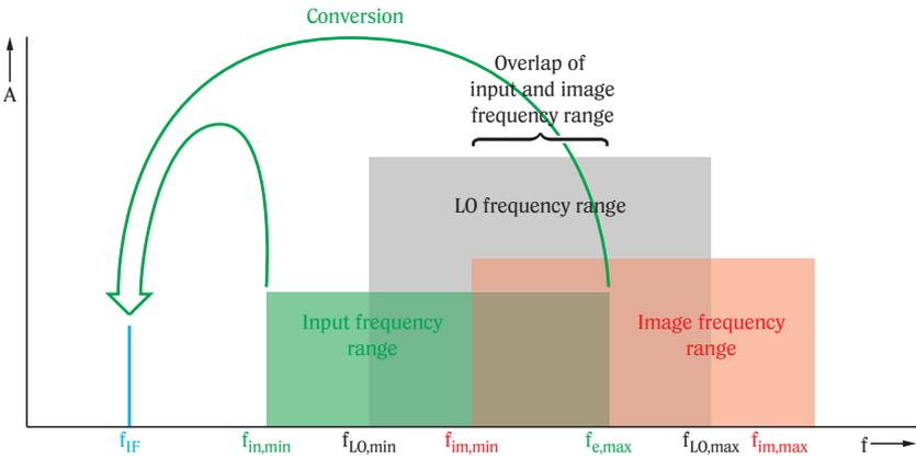
Fig. 4-3 Input and image frequency ranges (overlapping)
