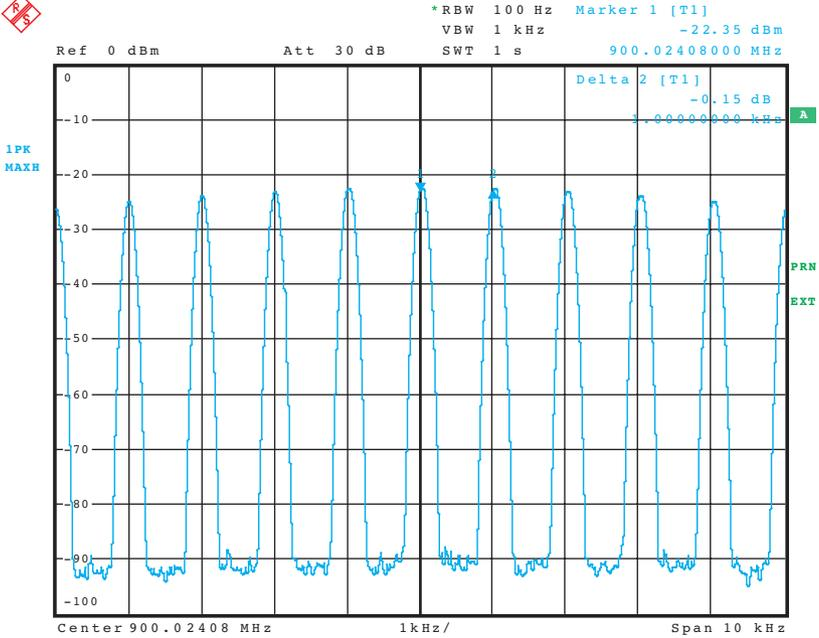
**Fig. 6-13** Line spectrum of pulsed signal
