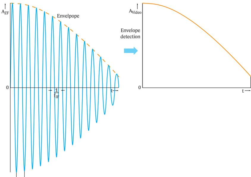
Fig. 4-15 Detection of IF signal envelope
