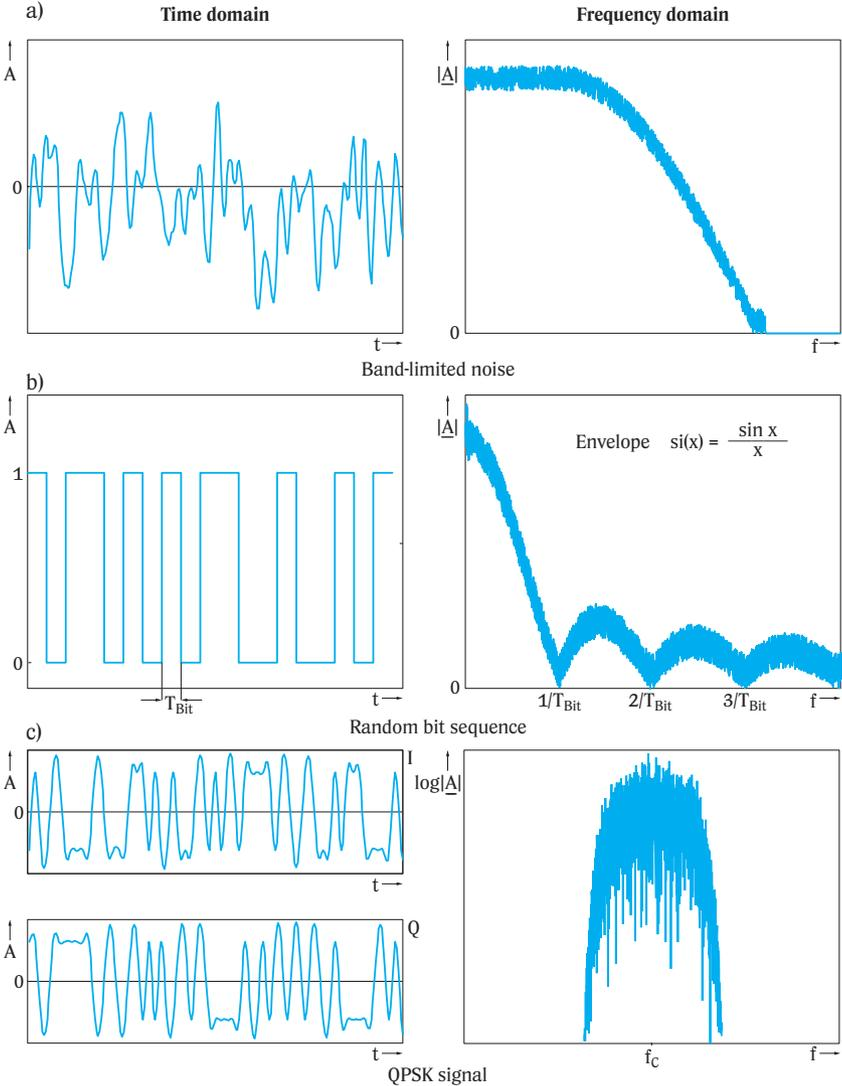
**Fig. 2-6** Non-periodic signals in time and frequency domain
