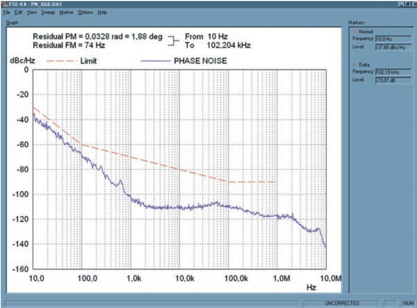
Fig. 6-3 Phase noise measurement over wide offset range
